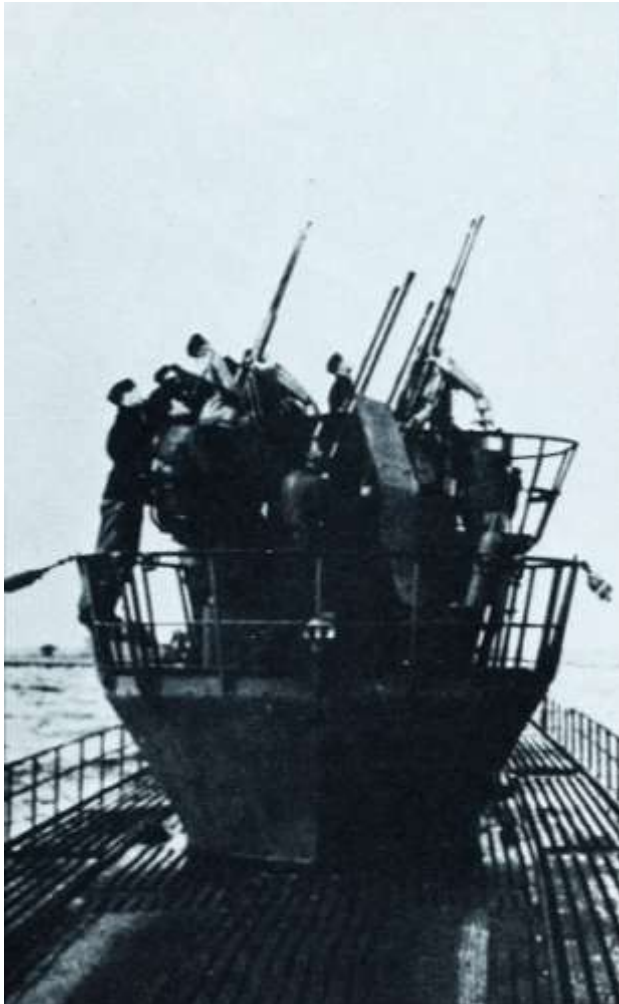
"Flak Trap". From mid-1943 in an attempt to give added protection against increasing numbers of aircraft attacks, U-boats were often armed with up to six 20mm quick firing canon in twin and quad mountings.
