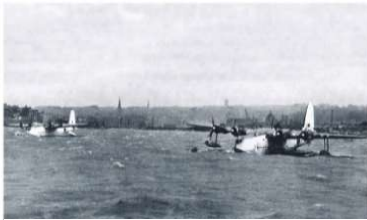
Two No.10 Sqn aircraft riding out rough weather in Plymouth Sound. Normal procedure required a skeleton crew to be on board to run the outer engines to prevent the aircraft breaking free from its mooring
